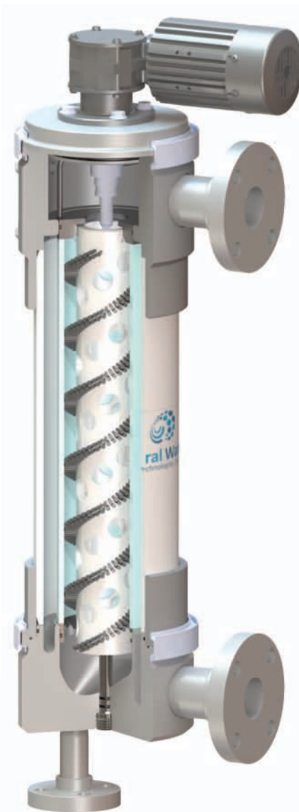
Spiral Water's Automatic Self-Cleaning Filter consists of a rugged stainless steel filter screen and a spiral-shaped brush that continuously cleans the screen without any backflush, crossflow or downtime.
