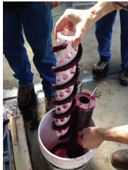
Spiral Water's unique action filters pomegranate solids, protects flavor
