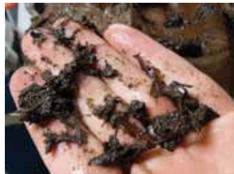
4: The bag-clogging debris filtered from the river water
