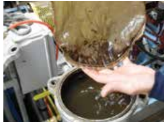
3: The filter bag used to protect the cooling water system
