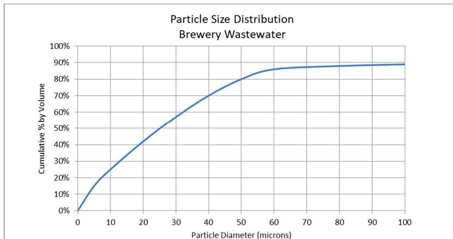
Figure 1. Particle Size Distribution of Brewery Wastewater.
