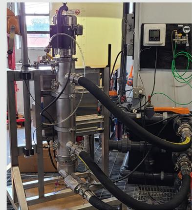
**Our Model 850 Automatic Filters**, available in stainless steel or PVC, is the latest evolution of our widely used Series 800 filters – our most compact product line, designed for lower flow, low pressure, low temperature applications.
