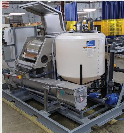
**Our break-out High Solids Water Recovery (HSWR) System** is a packaged, turnkey system that combines our Series 1000 automatic, self-cleaning filters with other industry equipment in various configurations depending on the intended application.
