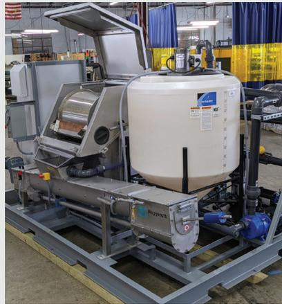
**Our break-out High Solids Water Recovery (HSWR) System** is a packaged, turnkey system that combines our Series 1000 automatic, self-cleaning filters with other industry equipment in various configurations depending on the intended application.
