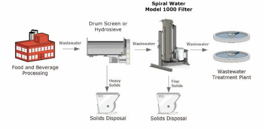
Wastewater generated by the food & beverage industry presents special challenges to wastewater treatment plants. The high levels of TSS, BOD, and fats, oils and grease are costly to treat. And while pretreatment to remove TSS and BOD can reduce overall treatment costs to the food processing plant, the ability to perform treatment at these facilities has been limited due to the difficulty of reducing TSS and BOD in a small footprint and at a low cost.
