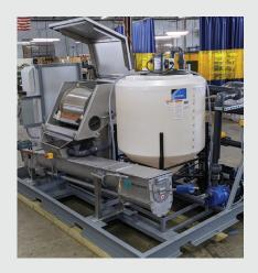
Water Recovery (HSWR) System is a packaged, turnkey system that combines our Series 1000 automatic, self-cleaning filters with other industry equipment in various configurations depending on the intended application.
