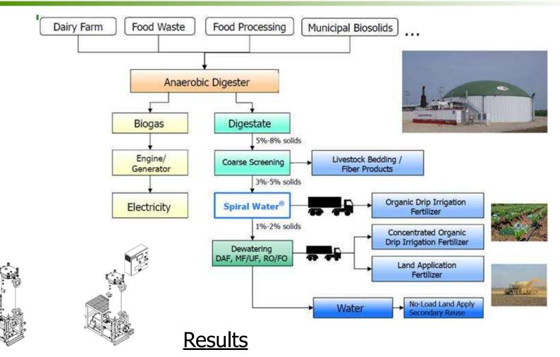
Installed Downstream of Digesters to Protect Membranes
